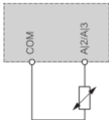
It is possible to connect either 1 sensors on terminals AI2 or AI3.
