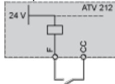
"PLC" position with PLC transistor outputs
