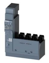
residual current device RCD110 basic RCD type A side mounted rated resid. current 0.03...5 A at 50/60 Hz tv instantaneous 4-pole In=160 A Ue=127-480 V accessory for: 3VM with terminal connection
