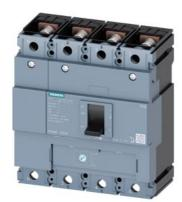
circuit breaker 3VM1 IEC frame 250 breaking capacity class S Icu=36kA @ 415V 4-pole, line protection TM220, ATFM, In=250A overload protection Ir=175A...250A short-circuit protection Ii=10 x In N conductor unprotected nut keeper kit
