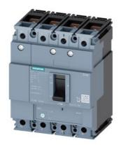
circuit breaker 3VM1 IEC frame 160 breaking capacity class N Icu=25kA @ 415V 4-pole, line protection TM220, ATFM, In=80A overload protection Ir=56A...80A short-circuit protection Ii=10 x In N conductor protection 100% nut keeper kit
