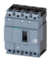
circuit breaker 3VM1 IEC frame 160 breaking capacity class N Icu=25kA @ 415V 4-pole, line protection TM220, ATFM, In=40A overload protection Ir=28A...40A short-circuit protection Ii=10 x In N conductor protection 100% nut keeper kit
