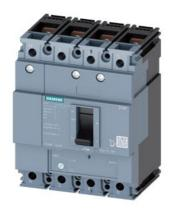
circuit breaker 3VM1 IEC frame 160 breaking capacity class N Icu=25kA @ 415V 4-pole, line protection TM220, ATFM, In=160A overload protection Ir=112A...160A short-circuit protection Ii=10 x In N conductor protection 100% nut keeper kit
