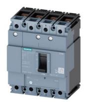
circuit breaker 3VM1 IEC frame 160 breaking capacity class N Icu=25kA @ 415V 4-pole, line protection TM220, ATFM, In=125A overload protection Ir=88A...125A short-circuit protection Ii=10 x In N conductor protection 100% nut keeper kit
