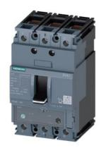
circuit breaker 3VA1 IEC frame 160 breaking capacity class S Icu=36kA @ 415V 3-pole, line protection TM240, ATAM, In=80A overload protection Ir=56A...80A short-circuit protection Ii=5...10 x In clamp connection
