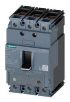
circuit breaker 3VA1 IEC frame 160 breaking capacity class S Icu=36kA @ 415V 3-pole, line protection TM240, ATAM, In=50A overload protection Ir=35A...50A short-circuit protection Ii=5...10 x In clamp connection
