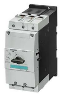
Circuit breaker size S3 for motor protection, Class 10 A-release 70...90 A Short-circuit release 1170 A Screw terminal Standard switching capacity !!! Phased-out product !!! Successor is SIRIUS 3RV2 Preferred successor type is >>3RV2041-4YA10<<
