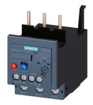
Overload relay 40... 50 A Thermal For motor protection Size S2, Class 10 Contactor mounting Main circuit: Screw Auxiliary circuit: Screw Manual-Automatic-Reset
