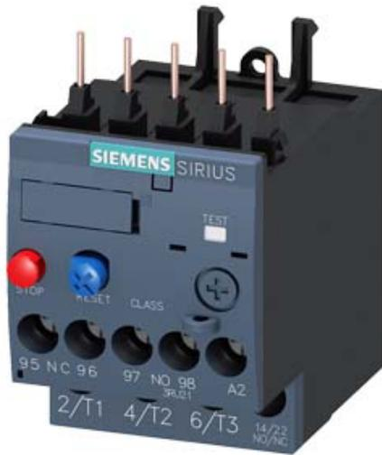
RELAIS DE SURCHARGE 9,0...12,5 A POUR PROTECTION MOTEUR BGR S00, CLASS 10 MONTAGE SUR CONTACTEUR CIRCUIT PRINC. : BORNE A VIS CIRCUIT AUX. : BORNE A VIS RAZ MAN-AUTO
