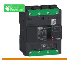
circuit breaker ComPact NSXm B (25 kA at 415 VAC), 4P 4d, 125 A rating TMD trip unit, EverLink connectors
