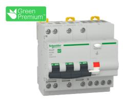
Residual current breaker with overcurrent protection (RCBO), Easy9, 3P+N, 25A, C curve, 4500A, AC type, 30mA
